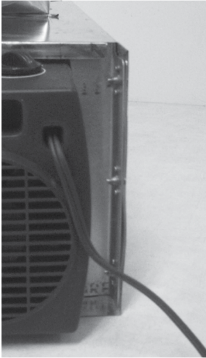
Above: view showing detail of the retaining angle trimmed to fit the curved side of the heater. Right, the end of the sheet metal box showing the stock end closeout riveted through the double folded end cap and the edges of the fabricated box
