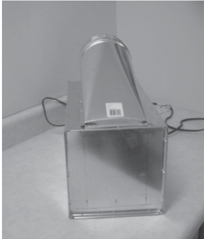
Left: opposite end view showing the stock end cap. Centre, end view showing Facto Heater with left and right side retaining pop riveted to the end of the fabricated heaterbox. Angle Brackets Trimmed to fit side contour of the heater. Right, the view showing the end close-out and top take-off.
