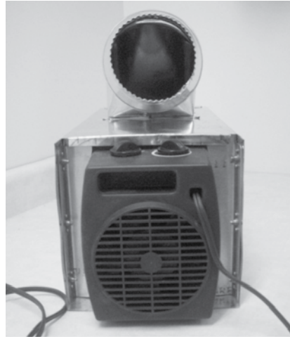
Left: opposite end view showing the stock end cap. Centre, end view showing Facto Heater with left and right side retaining pop riveted to the end of the fabricated heaterbox. Angle Brackets Trimmed to fit side contour of the heater. Right, the view showing the end close-out and top take-off.
