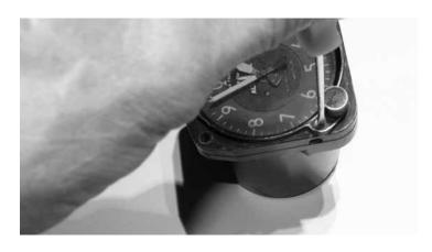
and the Kollsman window. This is as much as one should do to an altimeter. The accuracy required of an altimeter is in the range of 25 ft at low altitudes and 80 ft at 10,000 ft, and resetting the Kollsman does nothing to verify or correct accuracy throughout the range. The real question is, at one time the altitude and Kollsman presumably had correlation, so what happened to put them out of whack? If anyone knows, please email the office.
