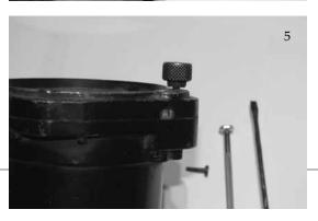
Above: Begin by setting the field elevation, then removing the brass screw that holds the lockpin. Fig 1: Look in the hole and you will see the threaded hole in the lockpin.
