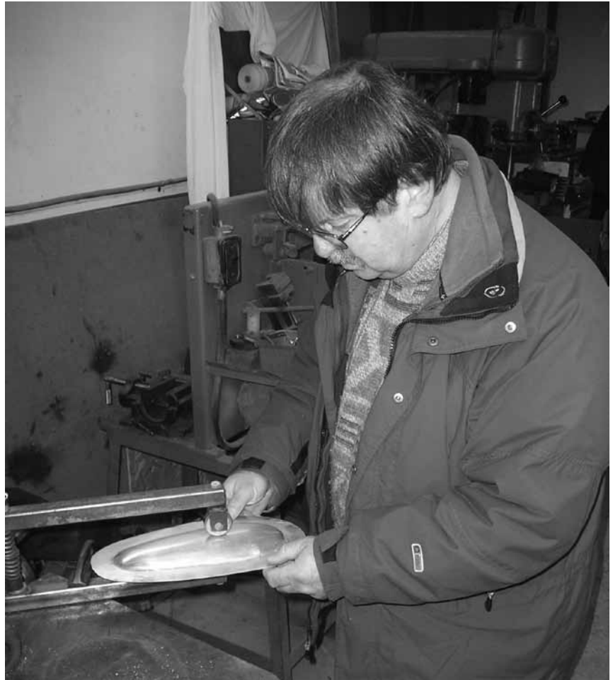
1: The pattern for the blister is cut out and taped to the plywood. 2: Establishing the size and shape of the aluminum blank. 3: The blank is bolted into the pattern. 4: The setup and tools used to form the blister. Above, the hammer marks are worked out with a small English Wheel. Opposite: the finished blister is now ready for trimming and fitting.
