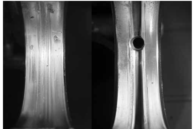
Left: The G-10 really is a small engine. The author's hand give a sense of its diminutive scale. Above, right: #4 Main bearing contamination.
