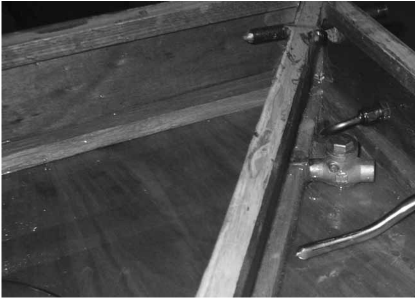
Above: The picture of the uncovered wooden gas tank shows most of the hardware involved. From the top; fuel filler, fuel drain, one of several check valves, fuel out to engine – this is the rear one, mechanical fuel gauge, and ground wire. Other stuff not shown here include pressure relief tubes between the sections and overflow drains.
