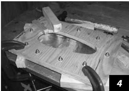
1: The pattern for the blister is cut out and taped to the plywood. 2: Establishing the size and shape of the aluminum blank. 3: The blank is bolted into the pattern. 4: The setup and tools used to form the blister. Above, the hammer marks are worked out with a small English Wheel. Opposite: the finished blister is now ready for trimming and fitting.
