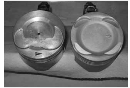
Left: the arrow points to oil supply for the turbo, immediately after the filter and from main galley. Inset: on the left, G10 piston and on its right, the G16 Vitara piston
