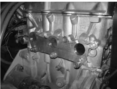
Top: The EGR Nozzle. Centre, the drilling jig used as a paint stand. Third down, NA rod and piston at top. Turbo / Gti rod on bottom, 19mm pin and 75mm Vitaro piston. Bottom, the intake manifold flange. Note that the injector bosses are not yet drilled.
