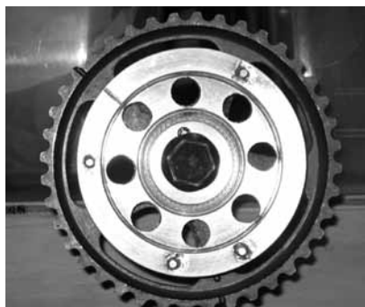
Simple Digital Systems G10 kit plus my own camshaft adapter
