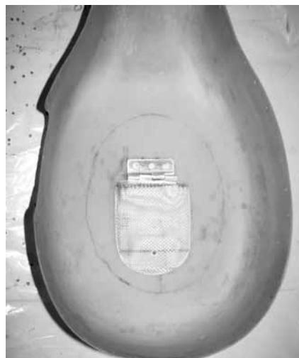
Left: The fiberglass reed is hinged on the inside of the airbox. If the main air passage becomes blocked the hinged reed will open to admit outside air. Centre: An aluminum bracket on the outside of the airbox has a hole for the spring that will pull the reed closed. ▶
